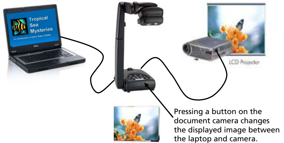
Figure 3. The manner in which the document camera “sits between” the computer and the projector, allowing the presenter to switch image sources by simply pressing a button on the document camera.
